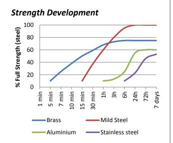
Cure times are typical at 23°C. Copper and its alloys will follow the faster cure while oxidised or passivated surfaces like stainless steel will tend towards the slower curve. Lower temperatures or large gaps will tend to extend the cure time. To reduce the cure time the use of Permabond A905, ASC10, or heat can be considered.
