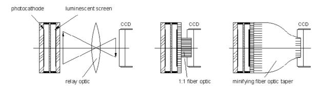
Transmission of the screen-picture to the image intensifier via a relay optic or via fiber optic coupling
